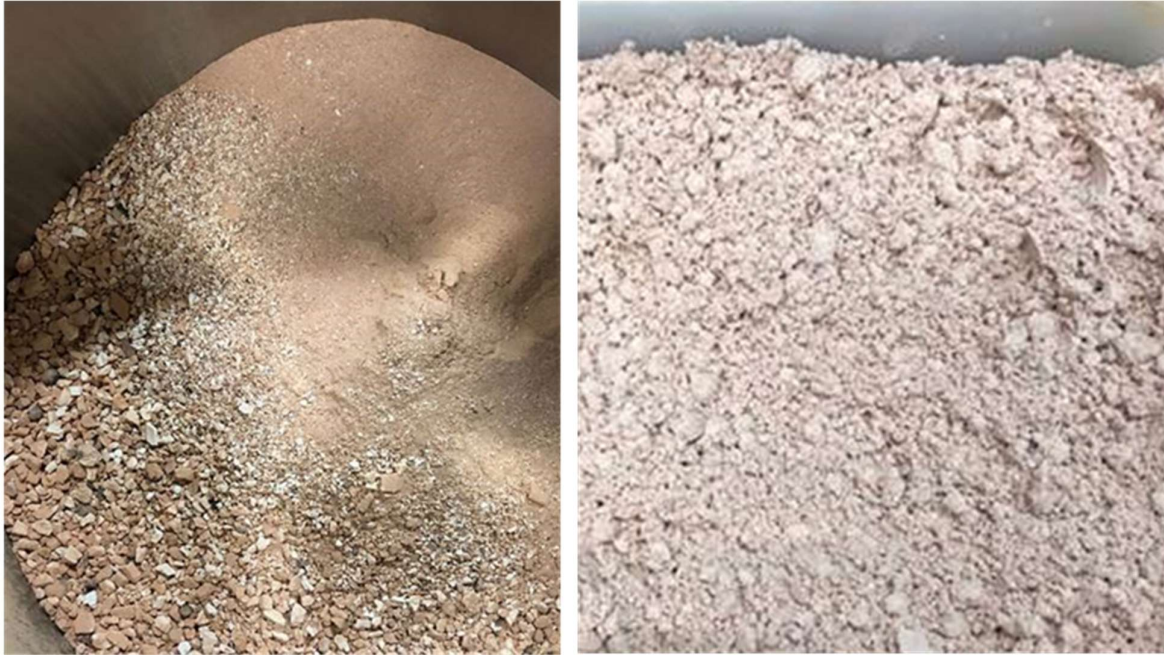
Figure 3 – Beta-spodumene product after calcination (left) and after milling (right)
