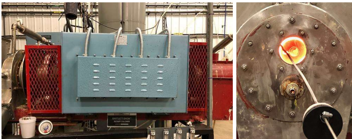
Figure 2 – SGS pilot kiln setup and calcination operation in progress
