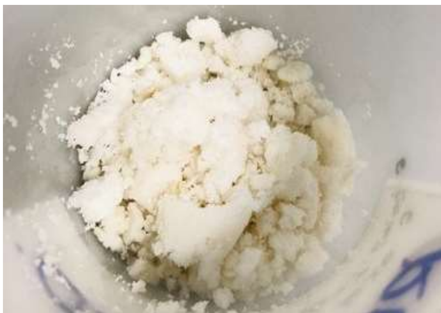
Figure 6 – Final Filtered 2 nd Stage LiOH Crystals
