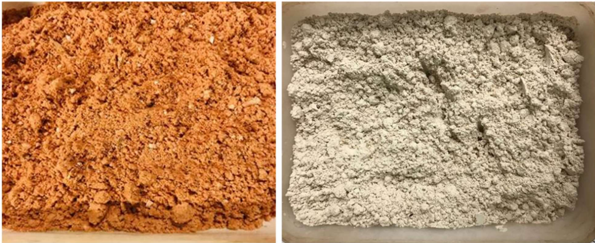
Figure 4 – Acid roasted calcined spodumene (left) and residual solids after water leach (right)
