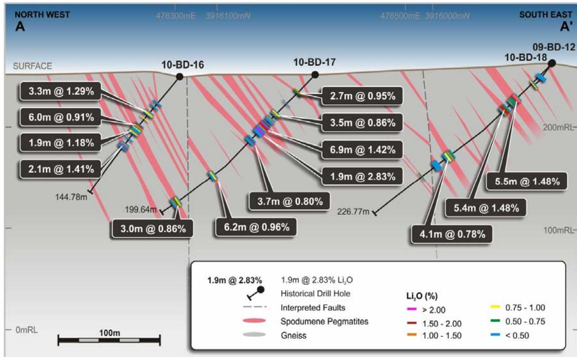
**Figure 3: Project Cross Section showing high frequency of Lithium Bearing Pegmatites**
